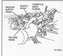
Fig. 11 Disconnecting the vacuum supply hose-4.6L engine
