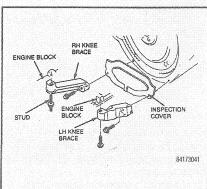
Fig. 14 Install an engine-lifting bracket at Fig. 13 Engine-to-transmission knee the front of the left cylinder head-4.6L braces-4.6L engine engine
