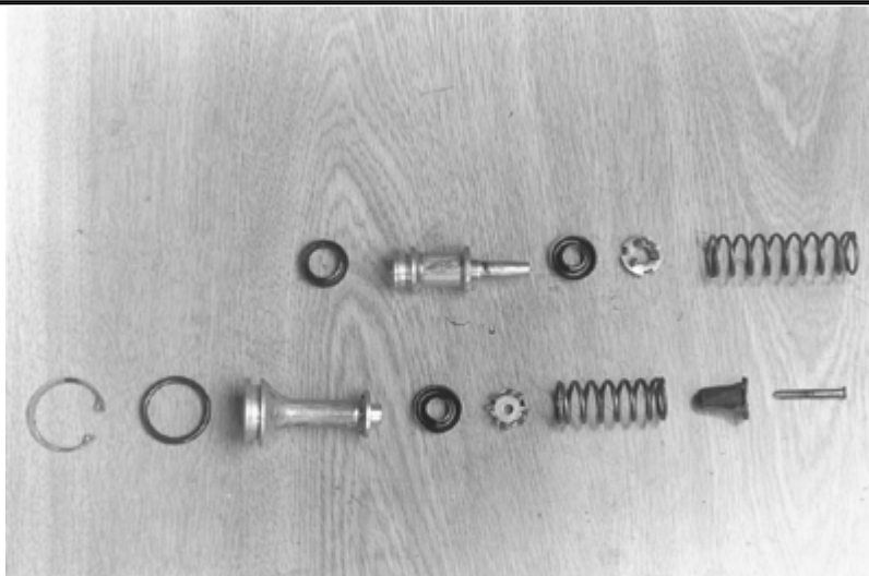
Exploded view of the internal components of the master cylinder
