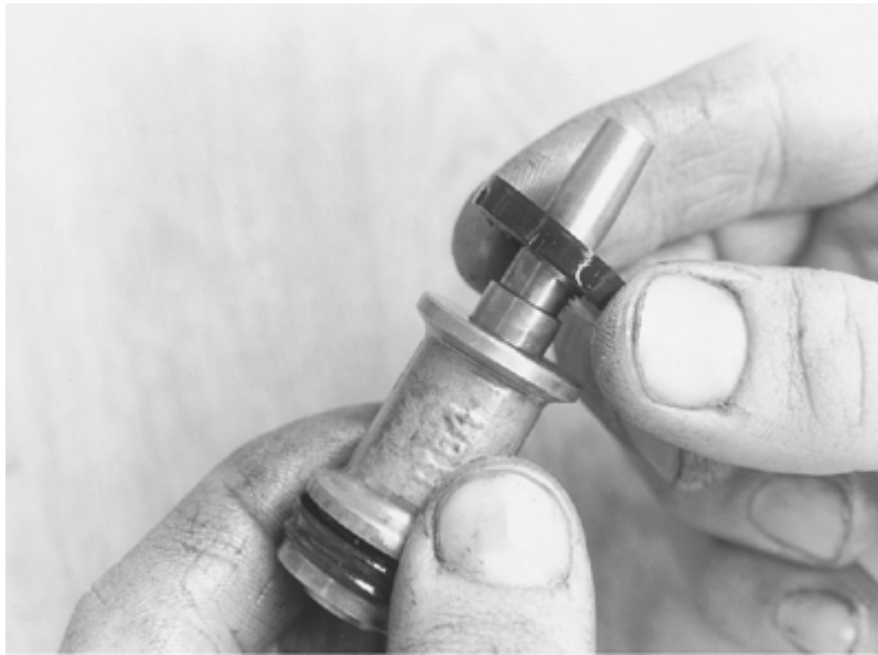
Replacing a seal on the secondary piston
