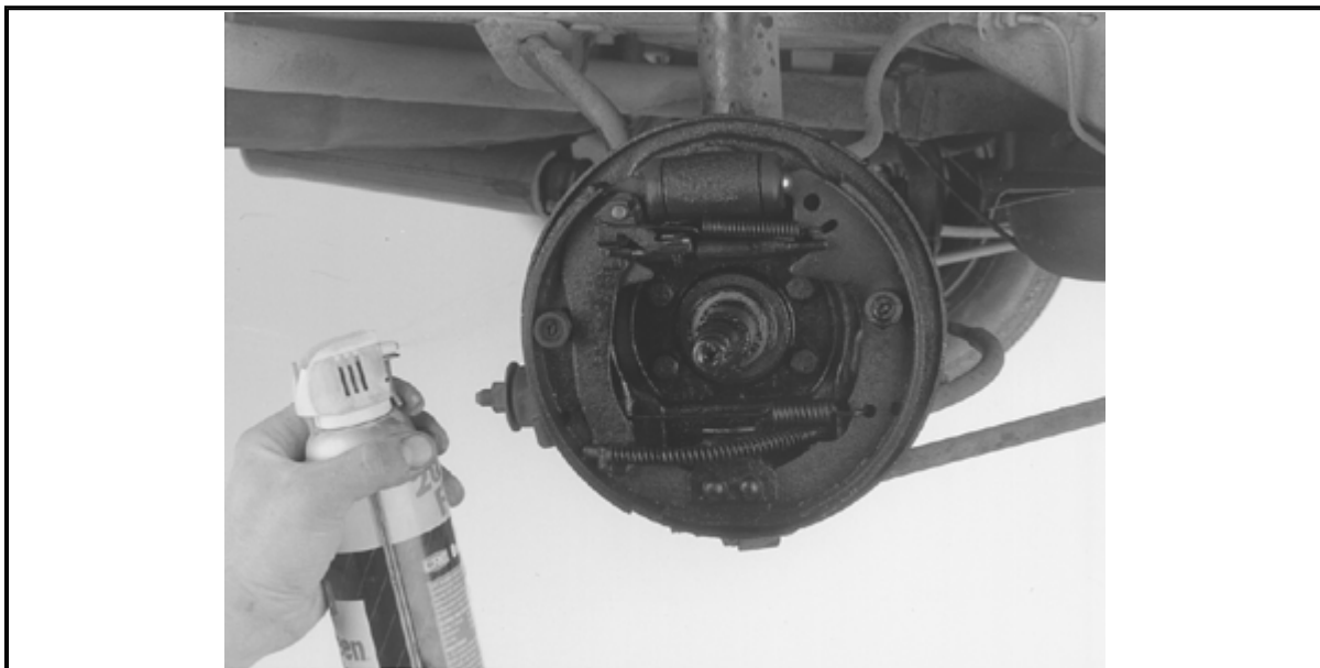
Use an evaporative spray brake cleaner to remove brake dust from the components
