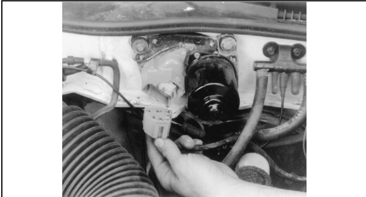
Disconnect the power lead from the windshield wiper motor
