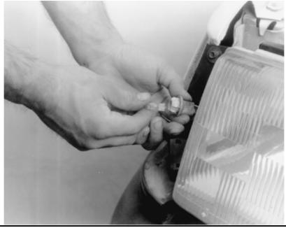
If the bulb needs to be replaced, remove it by pulling it straight out from the socket
