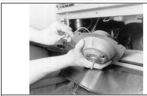
Remove the blower motor assembly from the vehicle
