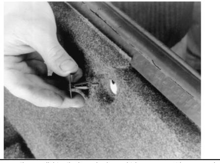
To access the rear lights, the lower back panel trim cover must be removed
