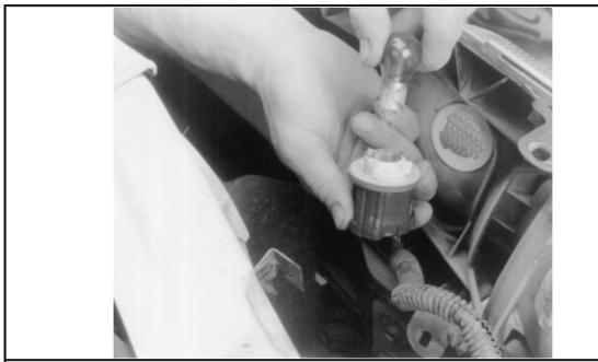
After removing the bulb/connector assembly, gently pull the light bulb from the socket for replacement
