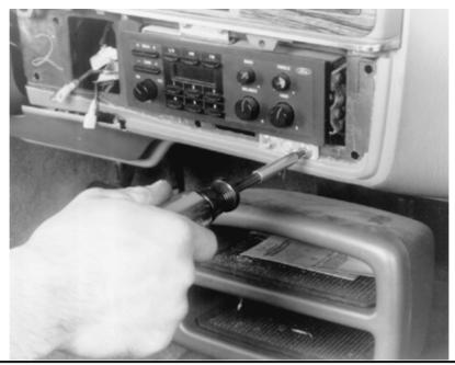
Remove the four screws retaining the radio and mounting bracket to the instrument panel
