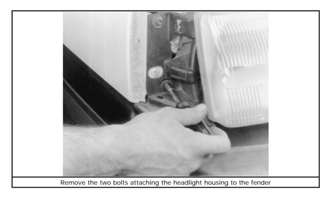
8. Remove the three bolts (Taurus) or four bolts (Sable) attaching the headlight housing to the brackets.
