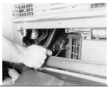
Remove the screws attaching the recirculation duct to the heater assembly, then remove the duct
