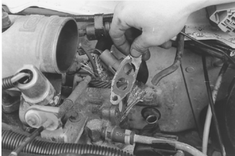
When installing the EGR valve, be sure to remove the old gasket and install a new one
