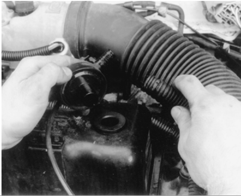
Disconnect the PCV hose, then set it aside-early model 2.5L shown
