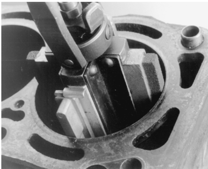
Removing the ridge from the cylinder bore using a ridge cutter
