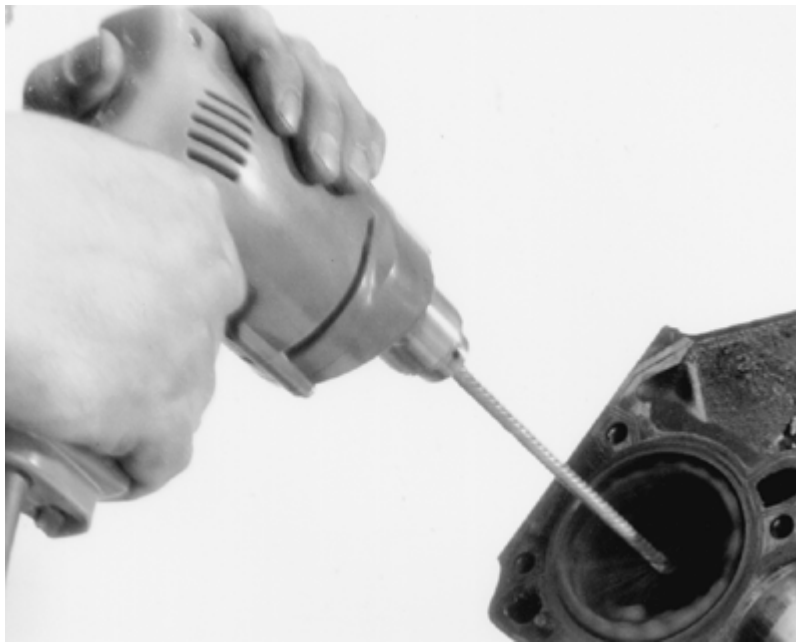
Removing cylinder glazing using a flexible hone
