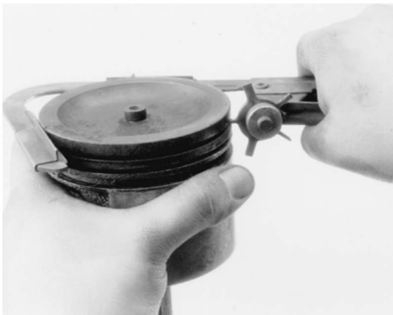
Clean the piston grooves using a ring groove cleaner
