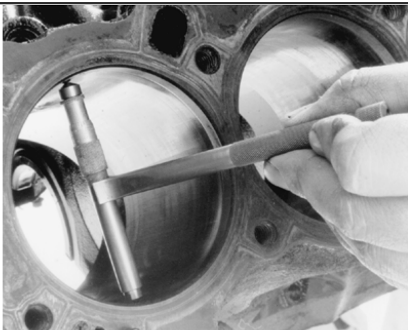
A telescoping gauge may be used to measure the cylinder bore diameter
