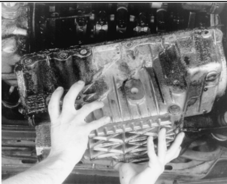
Carefully lower the oil pan from the engine
