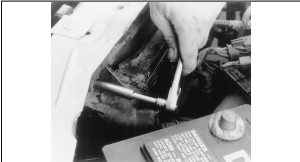
Remove the radiator retaining bolts/screws
