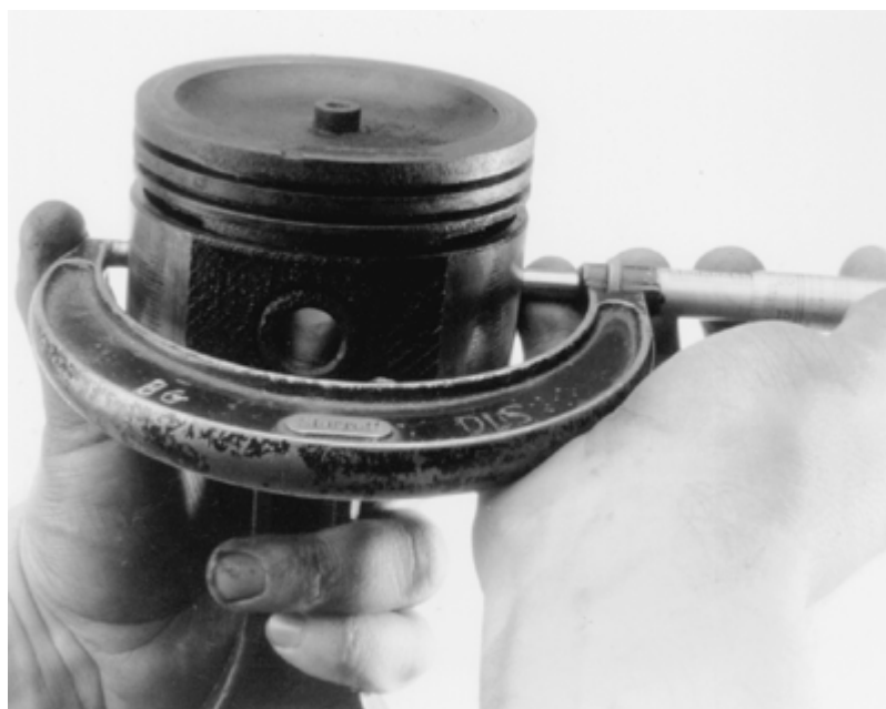
Measure the piston's outer diameter using a micrometer
