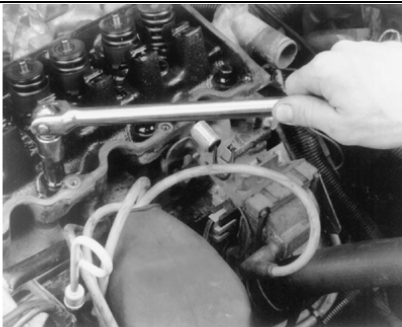
Removing the cylinder head bolts-2.5L engine
