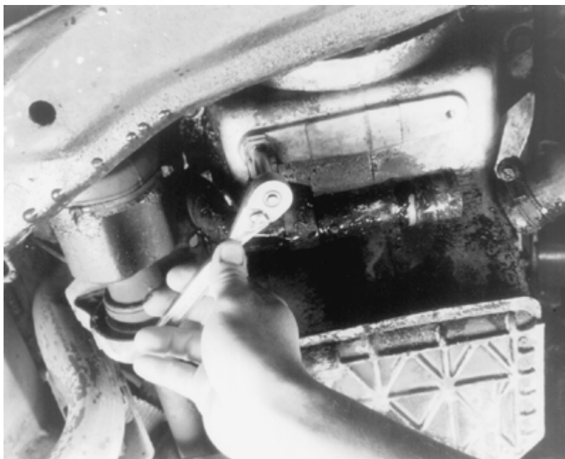
Remove the coolant tube-to-oil pan retainers, then...
