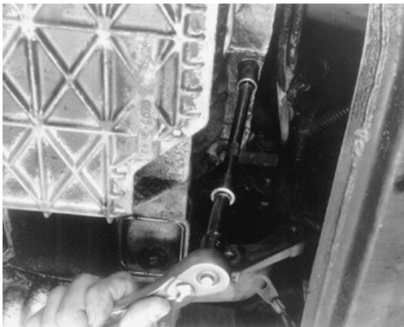
Remove the oil pan retaining bolts
