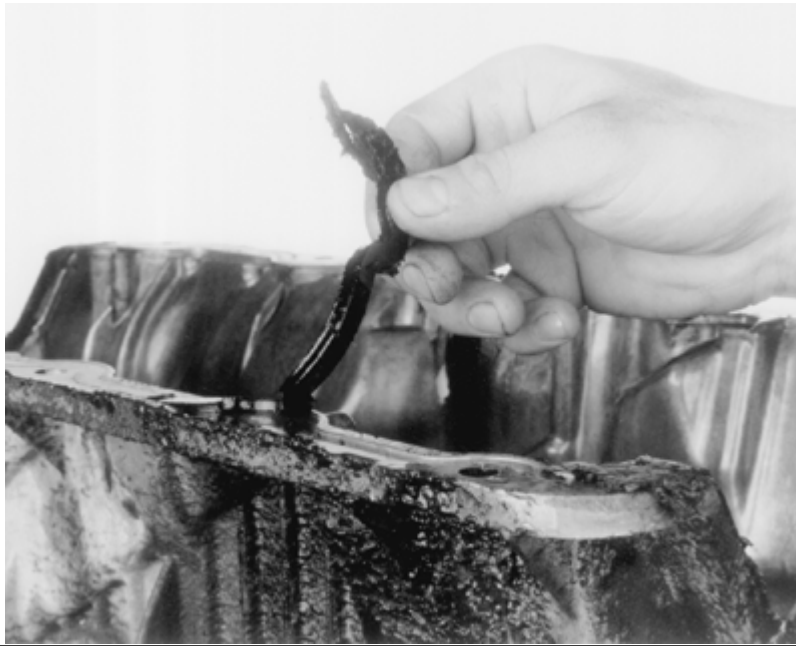
Clean all traces of gasket/sealer from the oil pan
