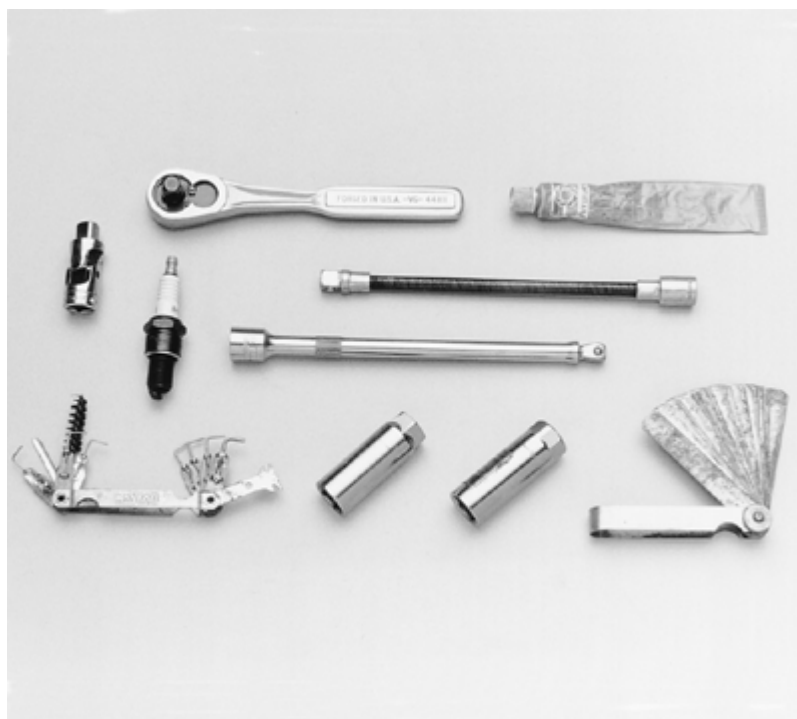
A variety of tools and gauges are needed for spark plug service
