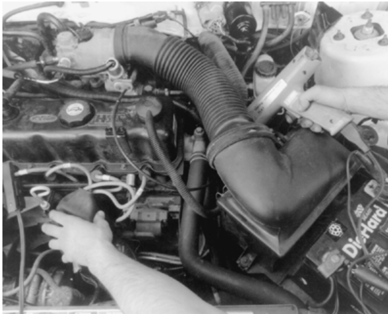
After the distributor is installed, check the timing with a timing light
