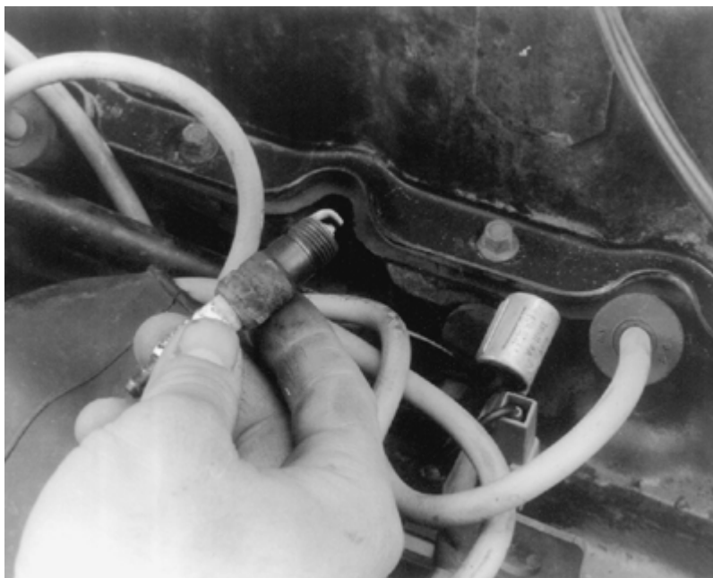
Inspect the plug for signs of fouling or deposits
